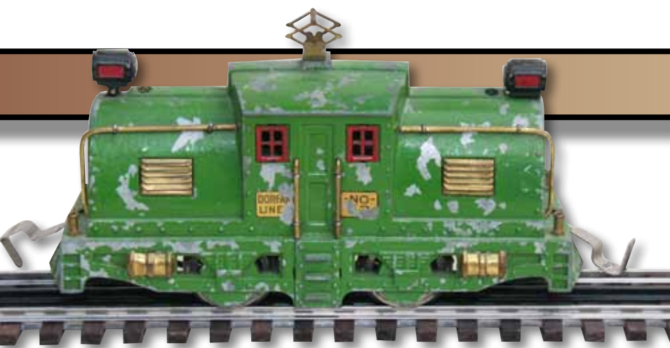
Photo 7 As far as other versions of the bipolar, I offer an interesting sample of Dorfan's work. Photo 7 is a Dorfan #53. Yes, that is a Lionel pantograph. I haven't found a repro Dorfan piece. It's a rather nice-looking engine, but it has a couple of problems common to Dorfan. One is that if I sneeze on it, the paint flakes. But the big problem is
