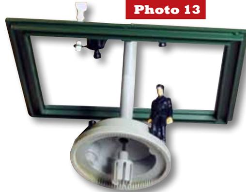
longer attached to the platform with the men. Instead, it is turned separately by the center gear seen in **photo 12**. The platform is turned by the secondary gear. What this does is turn the men in a clockwise direction and the rod in the opposite direction – an interesting
