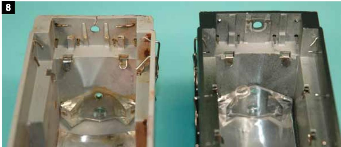
**Photo 8** illustrates the changes made to the male portion of the die to correct the problem. The postwar Lackawanna is on the left. As you can see, several changes were made. The area at the screw hole has been made thicker and the four vertical spacers have also been thickened and extended. I cannot verify exactly when these changes were made to the shell.
