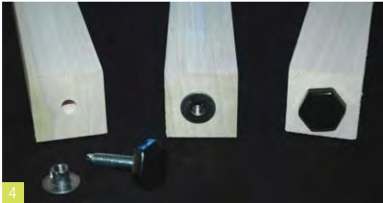
**Photo 4** shows the leg before installation, after the “T” nut is hammered in place, and finally with the leveler installed. The leveler allows an adjustment of up to 1-1/4 inches. The legs in my set were designed to make a table 36 inches high. Legs in several sizes up to 48 inches are available. Additional custom-made sizes are also available.
