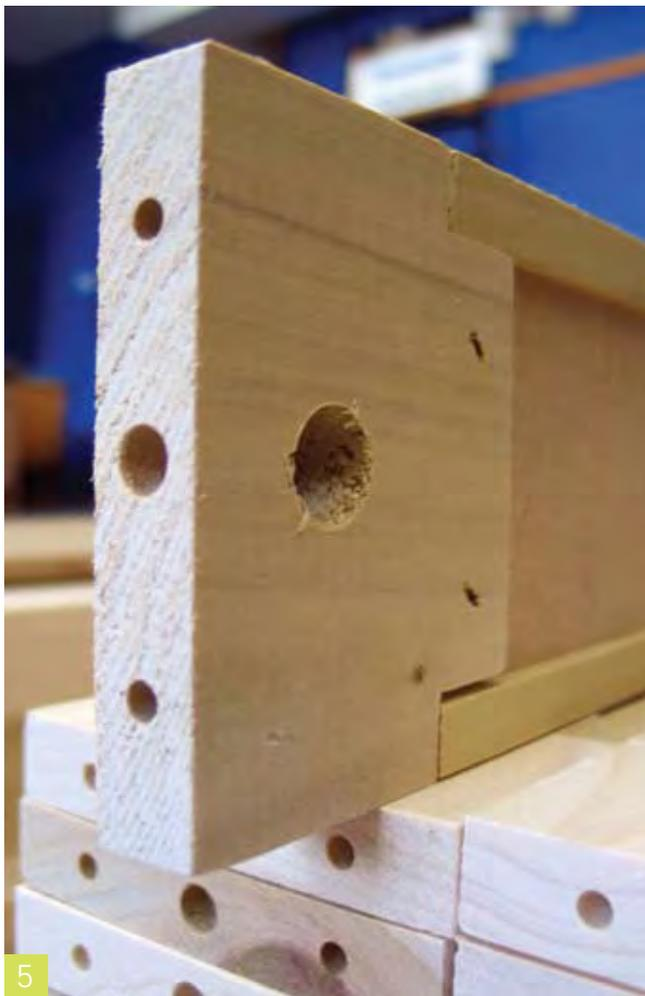
The beams which make the actual benchwork are unique in their design. Rather than solid wood, each beam is constructed with five pieces of wood. **Photo 5** shows the end of one of the beams. The center section of the beam is 1/4-inch medium density fiberboard (MDF). This piece is capped on its two long edges with poplar strips grooved to accept
