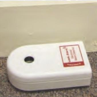
*Zircon Leak Alert™ Electronic Water Detector leaned against display shelves enclosing the layout tables. Except when being photographed, it lies flat on the floor either on its side or its back so that any moisture would establish a circuit between its two metal strip*
