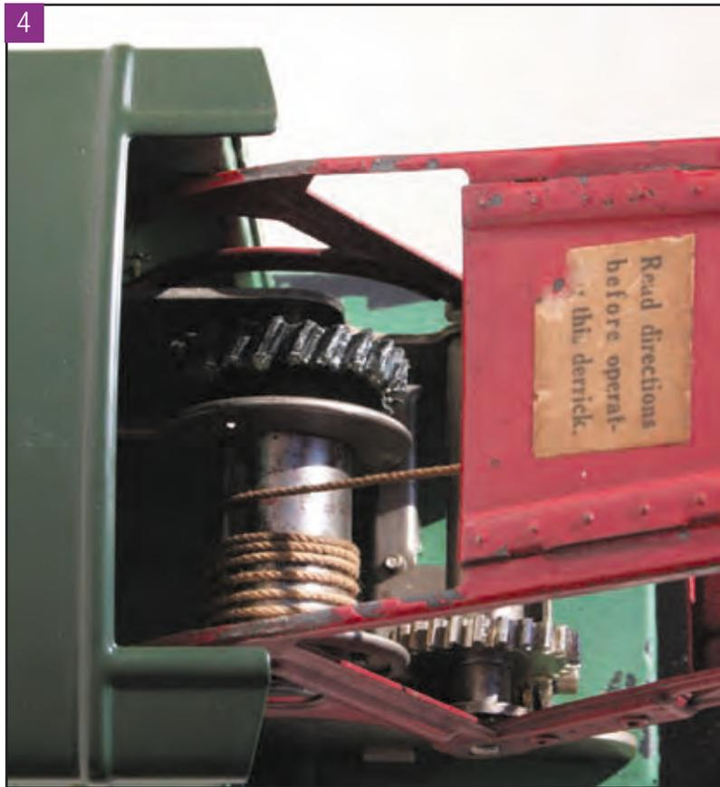
car body. The left one raises or lowers the hook, the right one the boom. See **photo 4** for a look at the gears inside the car body. Notice what big, solid gears they are. They are fine-tuning knobs; the gear ratios allow slow and precise motion in all three dimensions. No herky-jerky, coarse adjustments. When the big hook is called out to right the loco that spilled off the main, you need fine control. By the way, check out
