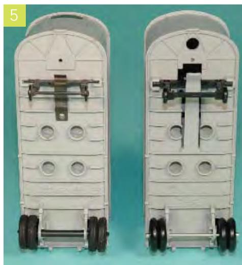
wheels. The original had a metal spring riveted in place to hold the die-cast pony wheels. The new version has an integral plastic spring clamp to hold the pony wheels which are plastic.
