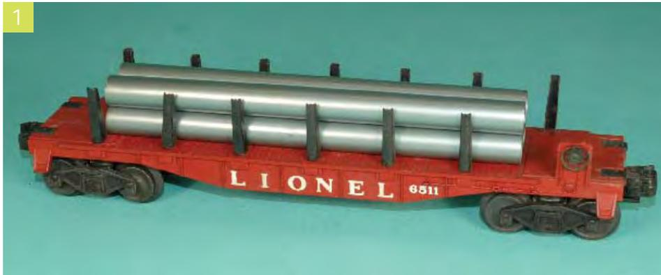
The flatcar on which this car is made became one of the most prolific for Lionel. The first appearance came in 1953 with the introduction of the 6511 Pipe Car. This new car was injection molded from plastic and offered "scale-detailing." **Photo 1** shows the original 6511 Pipe Car as it first appeared. When I first saw this car years ago, I was quite surprised to see how much the car had changed over the years. I was already familiar with the later versions of the flatcar produced in the 1960s.
