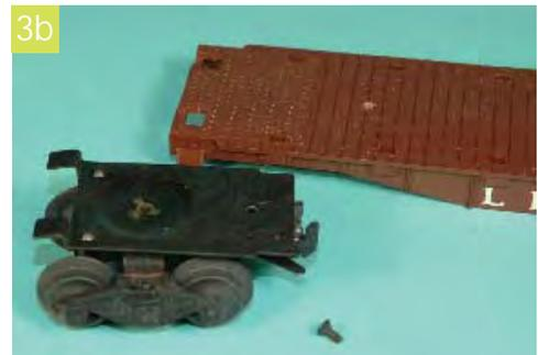
The method by which the truck mounted to the plate was also made more economically. No longer was there a post riveted to the truck. The "C" clip was replaced with a tubular mounting clip which was simply pressed through
