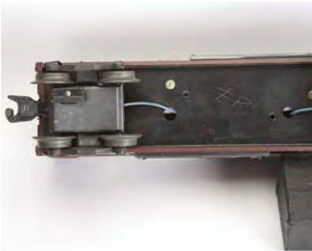
Note the underside of the frame for the tuscan #3454. Blue wire was typical for 1946 production and this particular frame has the etched initials "FP" which we assume is for Frank Pettit, a well-known, long-term employee of the Lionel Engineering Department.
