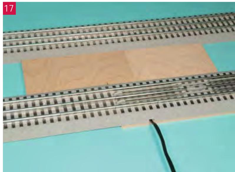
Now place the 10-inch section of the wood piece under the Remote Control Track and align it flush with that track section. The longer section of the wood will exactly space the parallel siding. See **photo 17**. I also placed an 1/8-inch shim under the track halfway between where the wood ends and where the track hits the table. This should be done on
