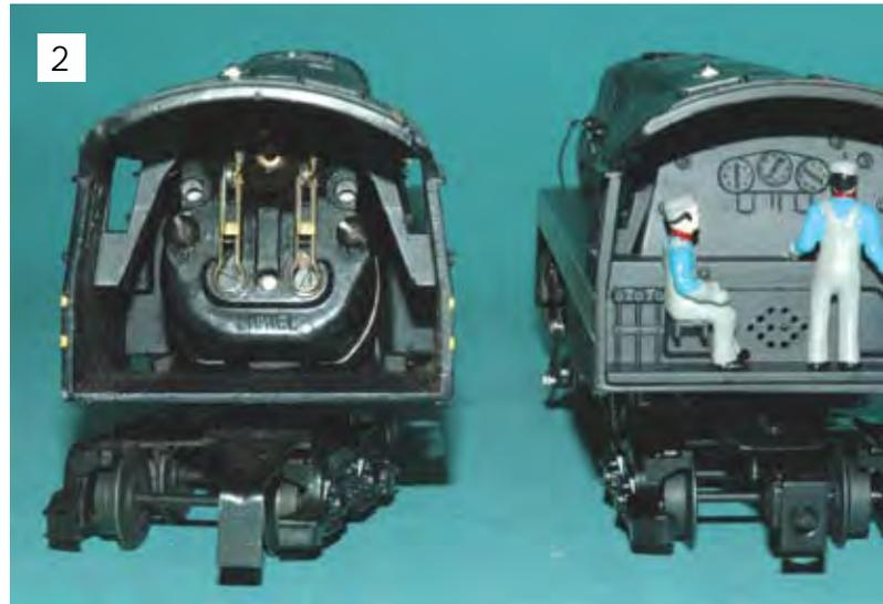
along with several visual improvements. **Photo 2** shows the cab of the original 746 on the left and the latest version on the right. Although the new one still features a Pullmor™ motor, it has been shielded with a detailed cab interior. It has a red firebox glow, and an engineer and fireman are on duty.
