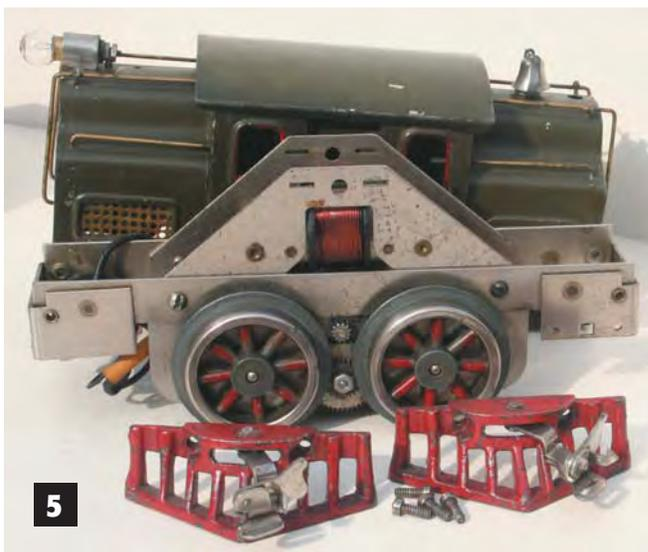
**Photo 5** shows the next version of the frame. This was used only for late production in 1923-24, and the body rides a little lower, which is why the frame can’t be seen when the body is in place. That’s one of the tip-offs that the olive green loco is later production than the black one.
