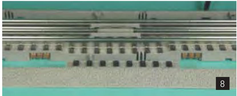
track is only five inches long, so additional rail sections are mounted to extend them to the full 10-inch length of the Operating Track. All three sections of the center rail have continuity to each other and all receive power.
