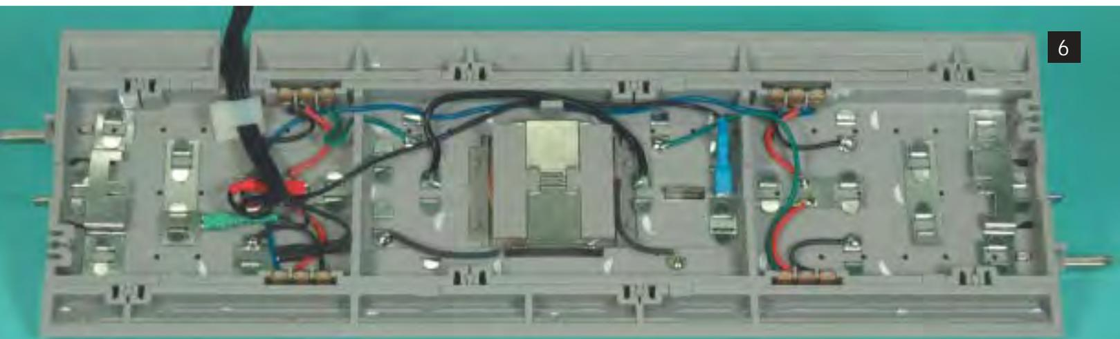
**Photo 6** shows its underside. The controller connections to the track are made with quick connectors and are color coded. In addition to the controller connections, there is other wiring — which is a complete mystery to me. Apparently those wires will be put to some clever use in the future. More on that later.
