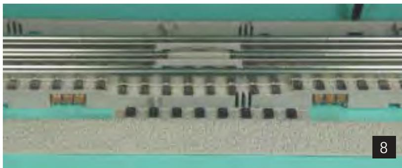
track is only five inches long, so additional rail sections are mounted to extend them to the full 10-inch length of the Operating Track. All three sections of the center rail have continuity to each other and all receive power.
