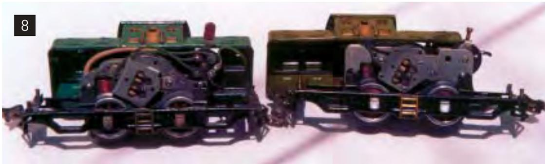
These locos also provide a bit of history of the development of motors. **Photo 8** shows the guts of the peacock 252. Both the shape of the motor frame and the brush plate mounting are the same as the last 150 series locos. Next to it is the olive 252. It has the same brush plate, but a newer, more rectangular frame. Look also at the hand reverse unit. That's the
