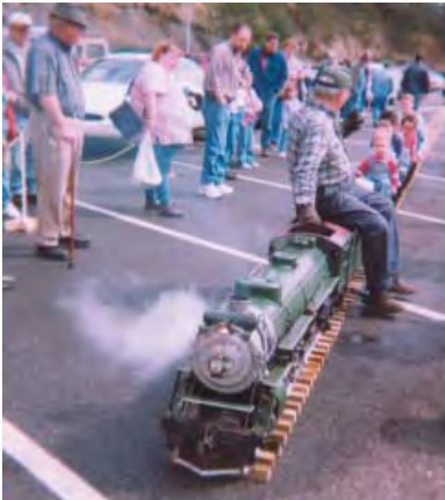
The premiere locomotive will be a Southern Crescent 4-6-2 in green and silver livery and trimmed in gold paint like the prototype. The locomotive is coal-fired, and its boiler operates at 80 to 120 pounds steam pressure. In operation, it consumes 10 gallons of water and burns about 20 pounds of coal per hour. The locomotive and its tender weigh nearly 900 pounds when empty.
