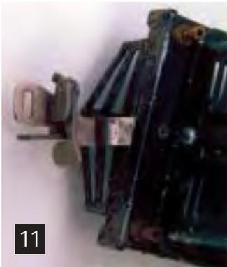
shot shows the transition coupler only available for a few years as Lionel moved from drop hook couplers to the "automatic" latch version. The slot is for the older cars. **Photo 12** shows it from the bottom. Essentially, it is a plate with a slot welded to the bottom of a latch coupler. I find these very useful when mixing equipment of different vintages.
