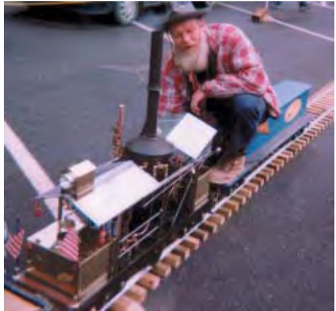
A second live steam locomotive — scratch-built, owned, and operated by Don Saager — will also be available for rides. A distinctive Shay logging locomotive with lot of side rod action, it was created from the plans of the prototype.
