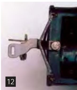
Essentially, it is a plate with a slot welded to the bottom of a latch coupler. I find these very useful when mixing equipment of different vintages.
