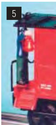
The movement of the original version was quick and snappy as one would expect with a solenoid. On Lionel's new version, the man moves slowly back and forth. His movements are continuous as long as there is power to the track on which
