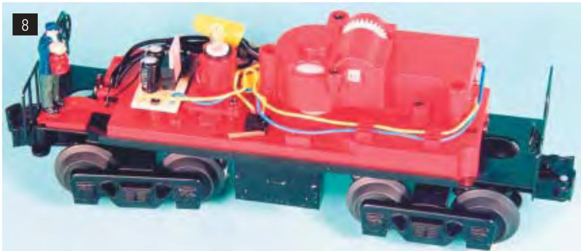
really no need to ever get in there. The large housing holds a small DC can motor and gear box assembly. The motor turns at high speed and the gears slow down its output and increase its power. The motor causes the arm on which the figure is mounted to move back and forth, slowly. There is no snap to the movement, but rather a more realistic continuous smooth back and forth motion.
