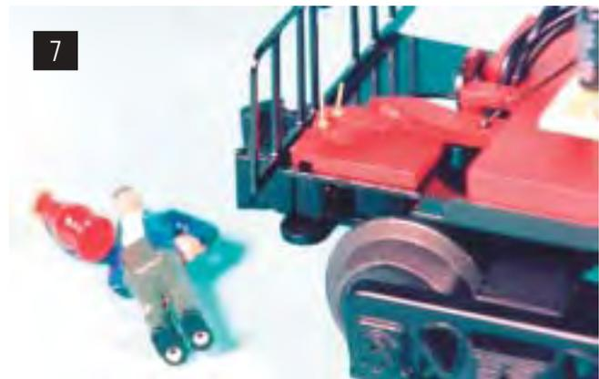
caboose. These pins carry current to the lantern held by the figure. The lantern is illuminated with a grain of wheat lamp. These last indefinitely and will most likely never need replacement. The lamp and its connections are molded within the figure. Should the lamp ever need replacement, the entire figure must be replaced.
