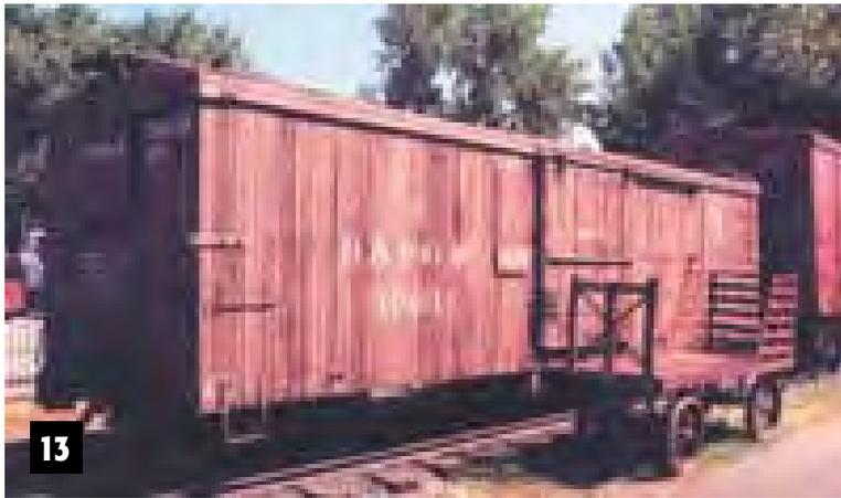
**Photo 13** shows narrow gauge D&RGW 23-ton capacity boxcar no. 3661 and was built in 1904. It hauled every imaginable commodity for over 60 years. You can see the difference in size between this narrow gauge car and the adjacent standard gauge size boxcar.
