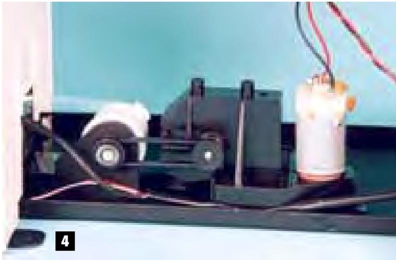
To view the motor, we first removed the two platforms. One screw in the center of the mill holds both of them in place. The opposite ends of these platforms are slotted and fit over metal tabs on the base plate. The left platform has wires and a small circuit board for the strobes and the DC motor. **Photo 4** shows Lionel's modern replacement for the vibrator motor. This rear view shows the motor and gear box driving the conveyor with a flat rubber belt.
