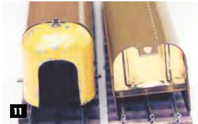
extension on the right of **photo 11** is simply dropped over the pin sticking up on the car in front and the rounded simulated vestibule does not pivot. Movement is strictly between the hole and the pin. **Photo 12** shows the complete Hafner train. The
