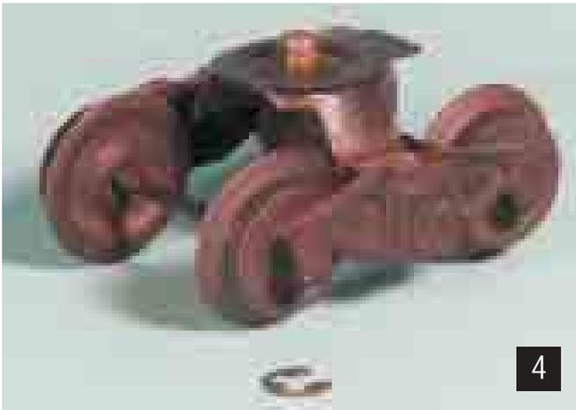
**Photo 4** shows the tender truck after the coupler has been removed. Notice also in the photo that one of the tabs on the top plate has been cut off. This is necessary to allow for clearance for the extended coupler. **Photo 5** shows the truck
