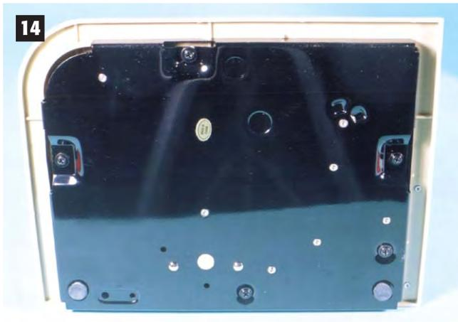
**Photo 14** shows the bottom of the latest version. Here you can see the five screws which hold the tan plastic in place. There is also the obligatory Made in China sticker. The base also has two rubber feet at the back edge and a third one centered towards the front.
