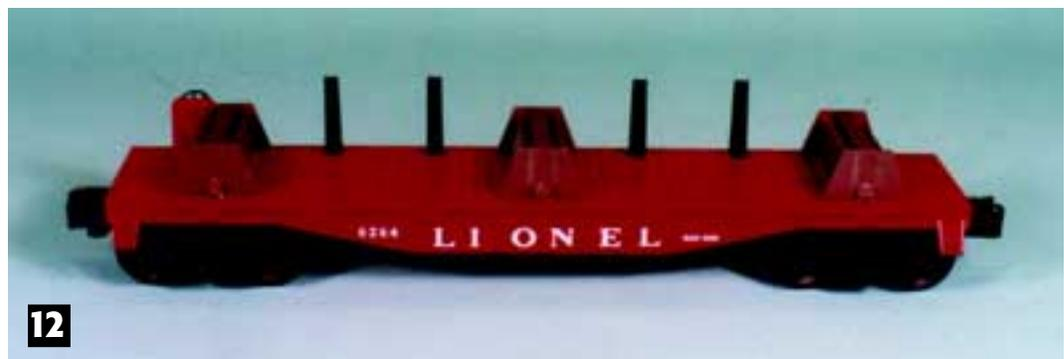
Personally, I'd rather have the die-cast version. The new version does away with the steel plate and the small square holes at each end on the top. The new version is equipped with die-cast sprung trucks. These trucks have done away with the plastic armature bar, substituting instead a steel bar and a machined steel button to replace the thumb tack. Bravo!!!
