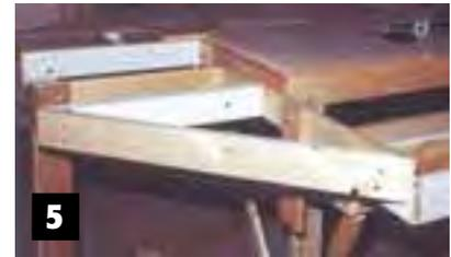
“Cascading frames” peripheral to the main level show benchwork for descending track.
