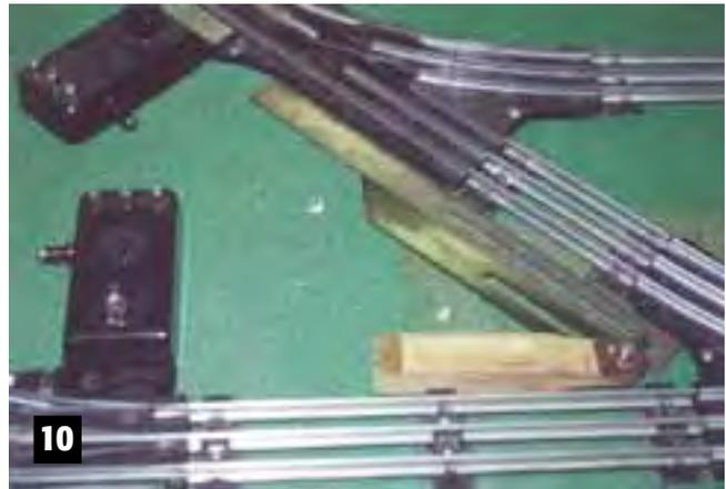
True Angle tool (set to 45°) can be used to set sidings in place at any desired angle.
