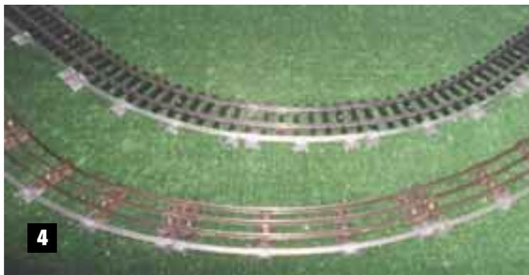
*Corners of track with an outside Lionel rail eased to a gauge of 3-3/8 inches so the rigid Buddy “L” cars can negotiate a 90-degree turn. An extra curved section of Lionel track has been inserted for standard gauge (front), but the G-gauge track (at rear) is already wide radius.*
