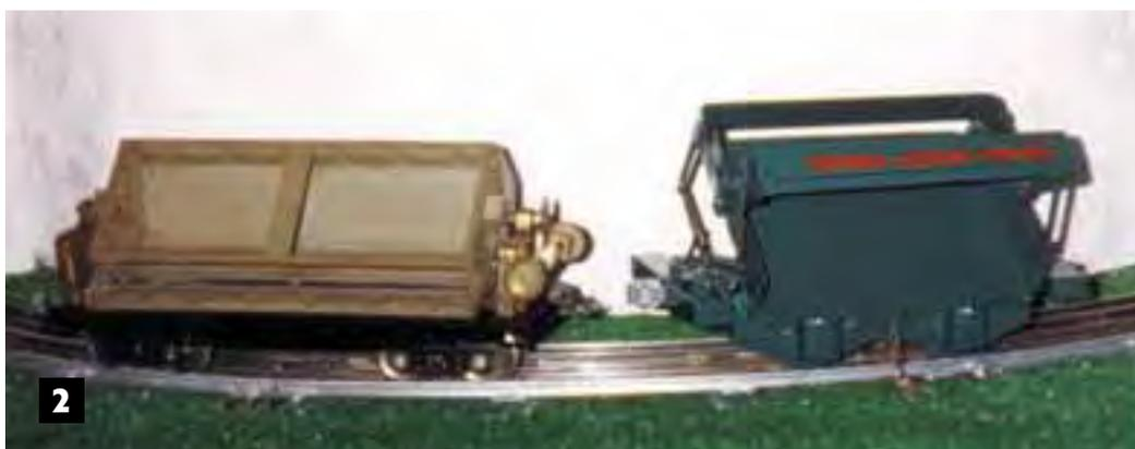
*The mechanism of the original Lionel 2-1/8-inch dump car (left) is a worm gear with two knobs on one end, while the Buddy “L” construction car uses levers to dump its load.*
