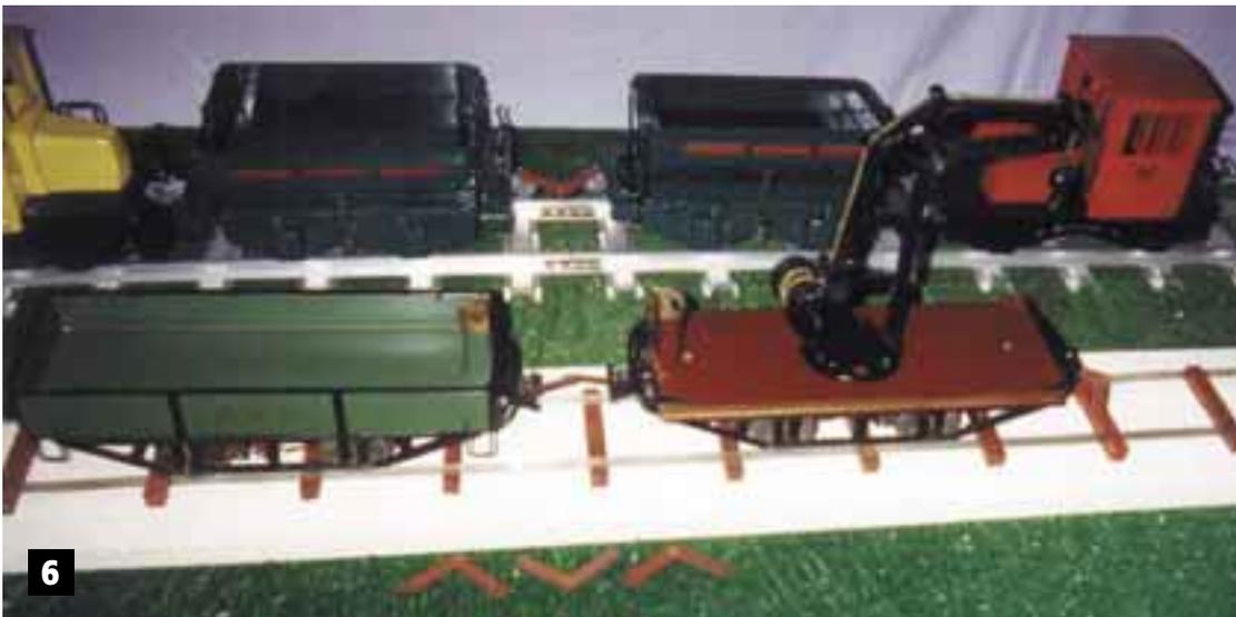
*Notice that the Lionel couplers for the 2-7/8-inch gauge train (foreground) can be used over the Buddy “L” knuckle couplers (rear) to solve two problems — they give incredible flexibility on curves and will not open.*
