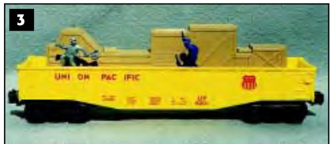
During the time when 9307 was being produced, a cheaper version was made for the Traditional Series of trains. In 1982-83 a yellow 6201 animated gondola was produced, see **Photo 3**. This gondola featured dual rubber band drive mechanisms with plastic wheels and trucks. The blue and gray rubber figures are unpainted and move around the unlettered tan crates erratically at best. The rubber band was wound around both axles on each truck and onto a spool at the center of the truck. The spools
