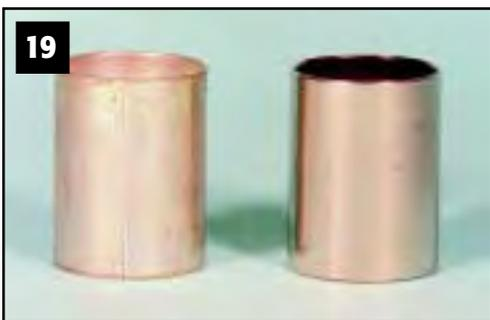
The new ones are slightly heavier and the seam has been welded and is not visible from the outside. The plating is also smoother and shinier.
