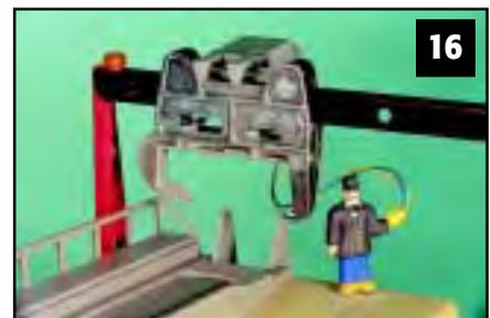
**Photo 16** shows the same view on the new version. The new version differs greatly from the original in that the motor driving the crane is mounted to it and travels with it. Power to the motor is carried through wires and a new Lionelville employee is in charge of holding these wires. The wires travel through him into the platform.
