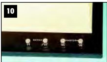
**Photo 9** shows the wire connections on the original version and **Photo 10** shows the new version with more desirable terminals replacing the clips.
