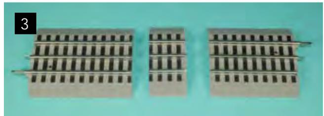
**Photo 3** shows the result. The very short middle piece can be discarded. Next I used a sanding block with 120 grit sandpaper and carefully smoothed the cut edges. Be careful not to sand it too much; all you want to do is remove the saw marks and leave a smooth, square edge for gluing. It takes very little sanding to achieve this. If you sand too much, you may lose the squareness of each piece and they will not mate perfectly. **Photo 4** shows the two cut edges after sanding.
