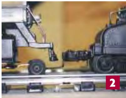
It is easy to fashion a little drawbar that hooks into that hole, carries a knuckle coupler on the other end, and couples with the tender in front of it for double-heading (see **photos 5, 6 and 7**).
