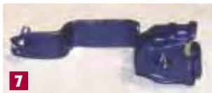
on the other end where indicated in the diagram, just big enough to thread the #4-40 1/4-inch machine screw securely into it. Fashion the little sheet metal plate that will go over the coupler opening (see diagram).
