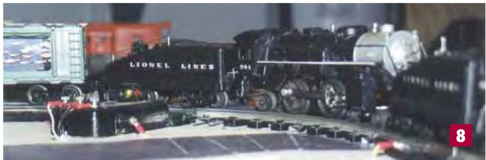
my tenders are spruced up with die-cast trucks, porthole lenses to fit on the backup lights, and handrails fashioned from some extra handrail wire — similar to those on the scale slope-back tenders.
