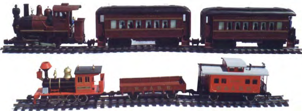
Modern trains of two different scales on the same 1-3/4 inch track. To the 1:22.5 Lionel “large scale” plastic passenger train on the upper level, the track is G metric. To the 1:32 Marklin Maxitrain on the lower level, the track is a standard gauge.
