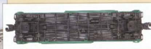
Separately applied metal underframe details
