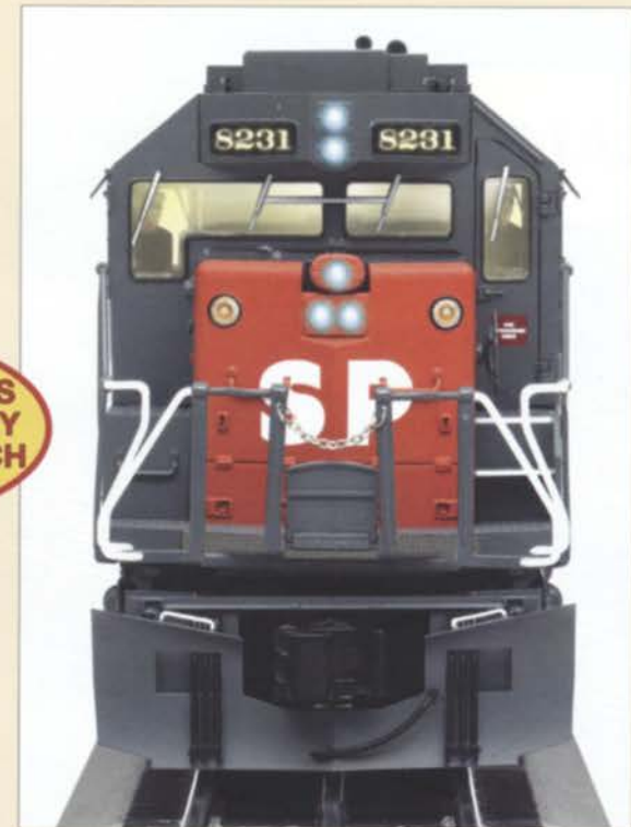
Prototypical headlight arrangement and “L”-shaped cab window
