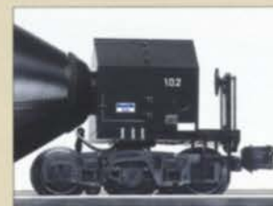
Fully equalized die-cast metal sprung trucks
