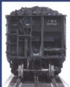
Die-cast metal end platforms
