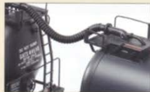
Separately applied valve details and flexible hoses
