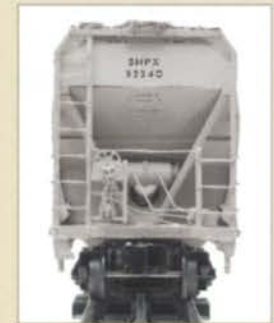
Die-cast metal end platforms
