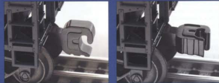
Realistic rotary couplers
