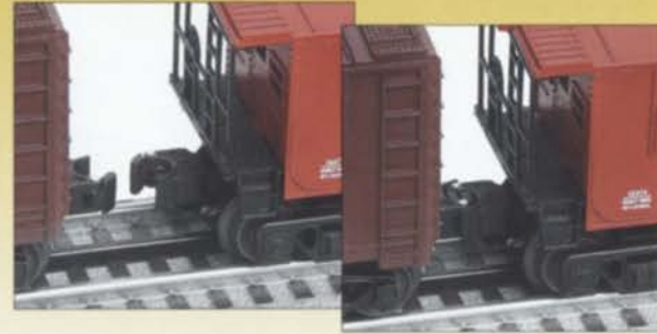
Realistic operating knuckle couplers
