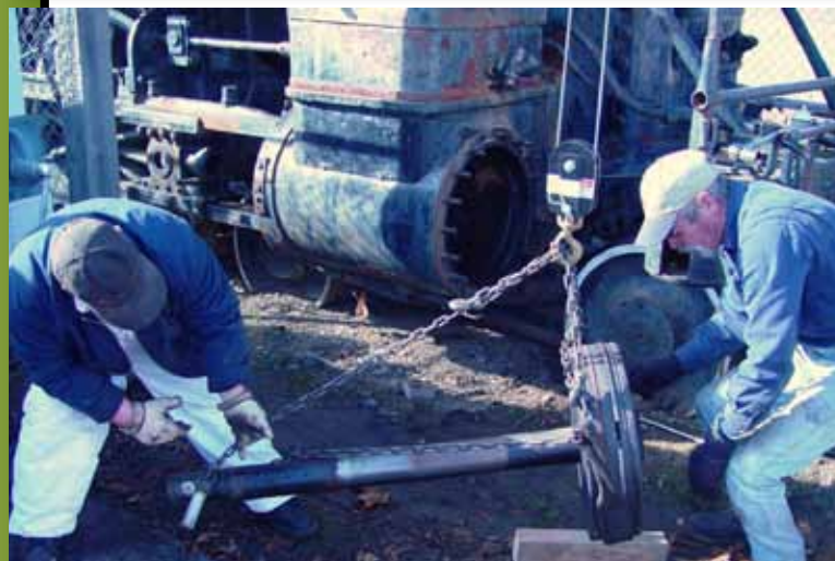
Removing the piston and rod from MoPac #2522 in Paris, AR.
