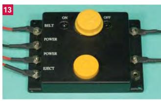
can activate the workman by pressing the lower button. The conveyor must remain on until the workman has moved the last can.
