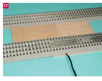
Now place the 10-inch section of the wood piece under the Remote Control Track and align it flush with that track section. The longer section of the wood will exactly space the parallel siding. See **photo 17**. I also placed an 1/8-inch shim under the track halfway between where the wood ends and where the track hits the table. This should be done on
