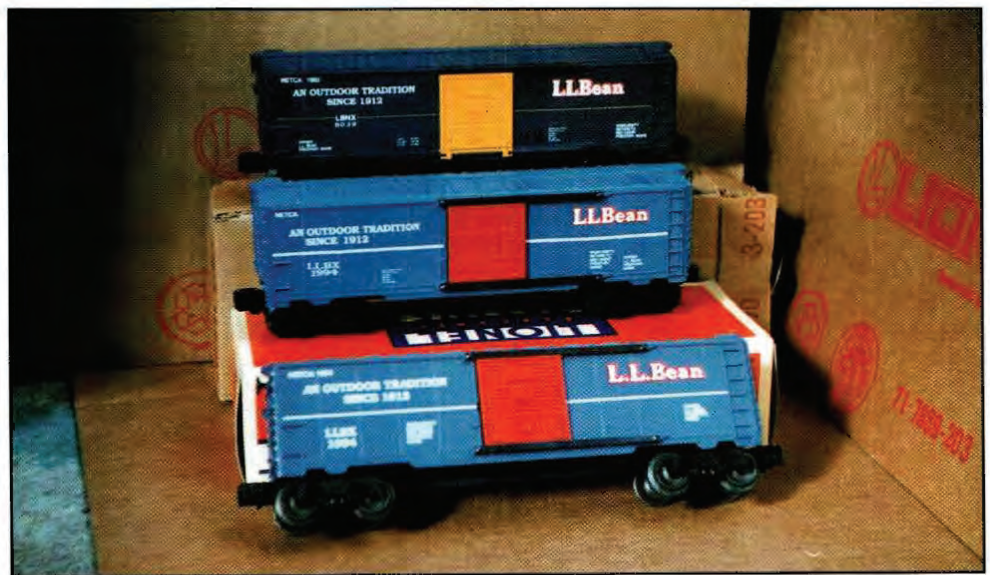
Photo shows at top, the first sample with yellow door; in the center, second sample with plastic trucks and the correct color combination but, no periods after the "L's" and; the final version with periods, metal door guides and sprung trucks. (Photograph by Ted Brahm.)
