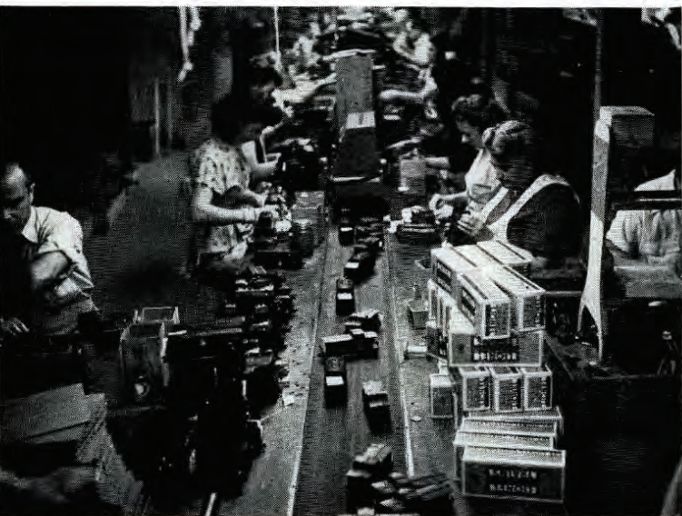
17 A production line of cars and tenders stretches out for nearly 100 feet and the light is supplied by fluorescent lights. These are so bright that they provided the only illumination for this picture. Other production lines make accessories, transformers, other cars and trucks.
