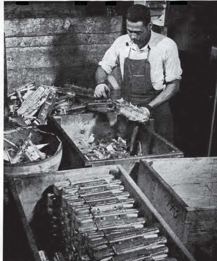
6 The excess metal must be cleaned from the die-cast bodies which will then be sent to other men who will grind and polish until surfaces are smooth and even and all edges cleaned of roughness. Although it is basically there, the GG-1 at this point lacks any handsome appearance.
