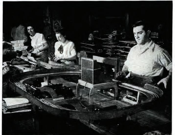
15 Another thing that amazes visitors is that at the last stage on the production lines, the engines run along on their own power. The little engine at the left will make a turn under the watchful eye of the inspector and then will run off to the left background for a final check.
