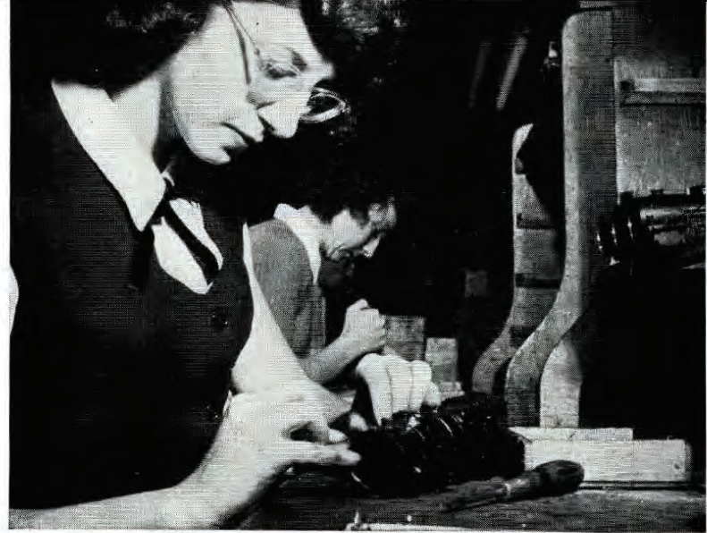
12 First step on the production lines is the adding of handrails, and then other details are added by some fifty workers on both sides of the moving belt. All small parts come from operations in the factory, and the motors are assembled on a different line and then inserted here.
