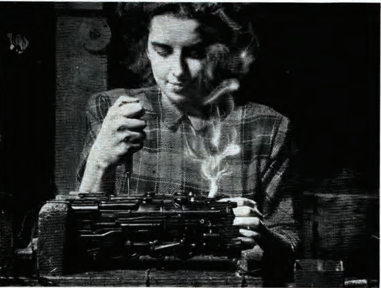
14 While adding a detail and tightening a screw, this girl checks the smoke and the running of the train in a special jig. As with all of the production line workers, her motions are quick, deft and sure. Special jigs make for easy handling of engines, even though they're heavy.
