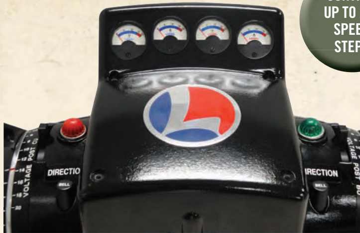
Clearly displayed voltage and current from each of the four channels.
