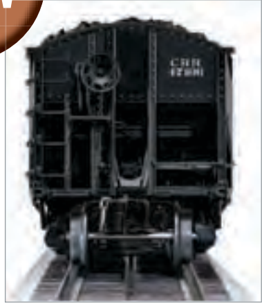
Prototypical curved ends on hopper
