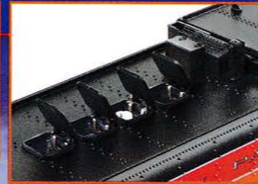
Opening tender water hatches reveal RailSounds controls
