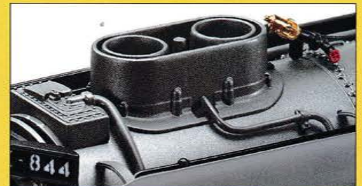
FEF-3 locomotives were delivered with twin stacks
