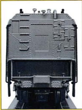
The FEF-3 class was delivered with 14-wheel "centipede" tenders
