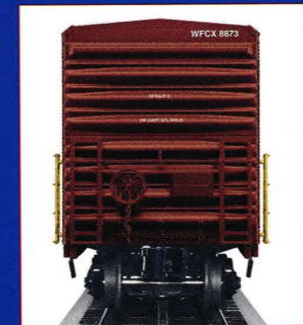
Separately applied details, including modern brake equipment and ladders
