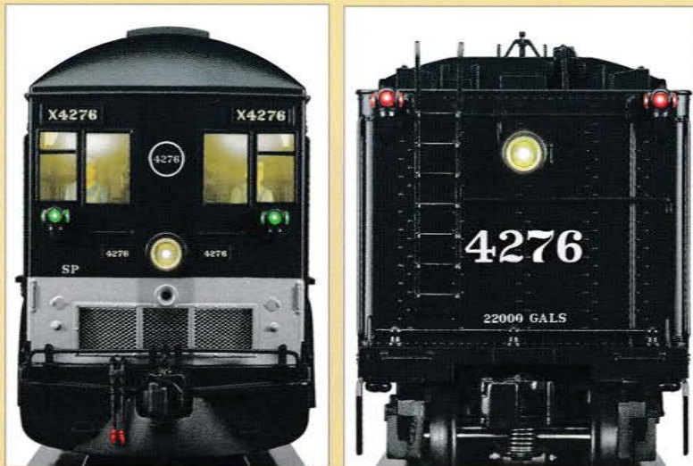
Directional lighting, including tender back-up light
