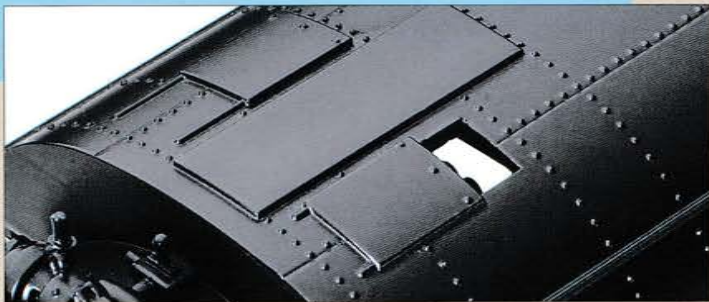
Opening roof hatches
