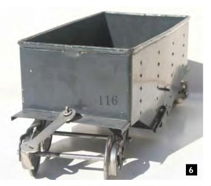
ones with rubber-stamping may have the catalog number 116 either at the end of one side or on the end of the car as shown in **photo 6**.
