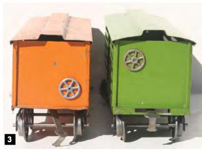
Brake wheels and coupler supports were like the 113s. **Photo 3** shows the brake wheels. I believe the wheels on this 114 are repros, but the placement is odd yet original. There are no plugged holes up high. I don't have a clue! This photo also clearly shows the difference between coupler supports and no supports. Coupler supports on both of these cars
