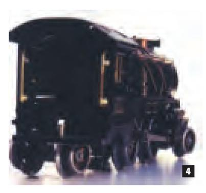
**photo 3**, the warpage in the longer section of frame is even more apparent by looking along it lengthwise, as in **photo 4**. You might want to add this "point of view" to your buying habits!
