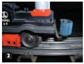
Photo No.2 shows the die cast platform support and the U reversing plate on the prototype.
