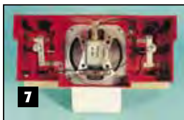
Photo 7 shows a view inside the original Station. The speaker was four inches in diameter. Two "D" cell batteries were held on each side of a threaded rod on
