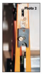
object right at the tip of the blue pencil is clipped to the belt assembly. The string is fastened to the bottom of this "spool." As the pulley drives the belt, the nylon line is made taught or slack as the belt travels in racetrack fashion.
