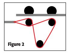
The part that passed under the first pulley passes over the second pulley, and then to the magnetic hoist. It is recommended that this line not be untied, but rather re-threaded if needed.
