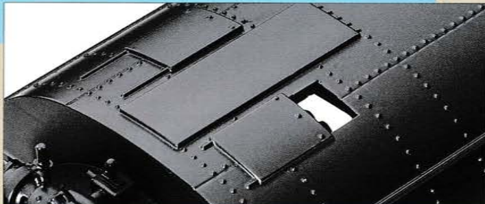
Opening roof hatches
