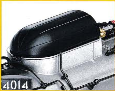
Smoke stack hood lifts away to reveal the double stacks
