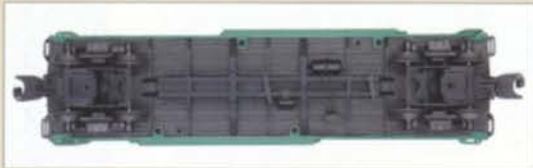
Separately applied metal underframe details
