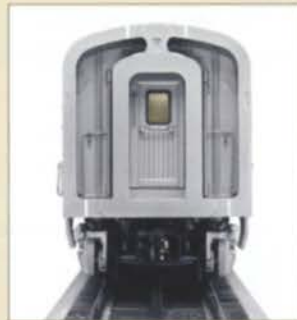
End vestibules with opening doors
