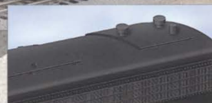
Exhaust stacks for steam boilers on FPA-4
