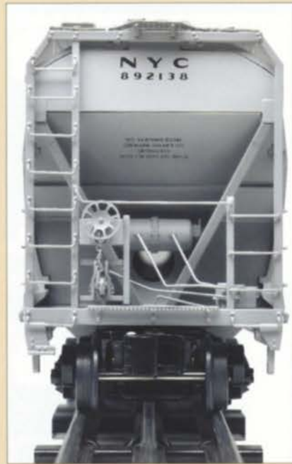
Die-cast metal end platforms
