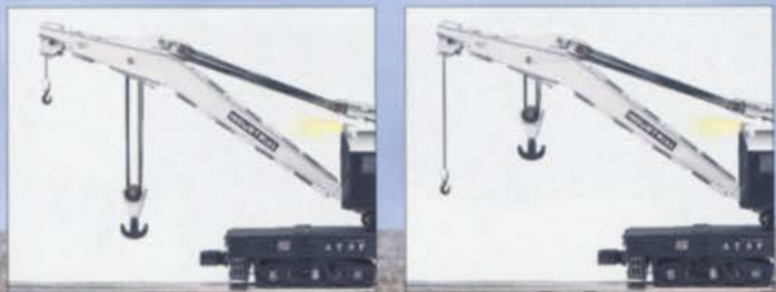
Independent control of main and auxilliary hooks
