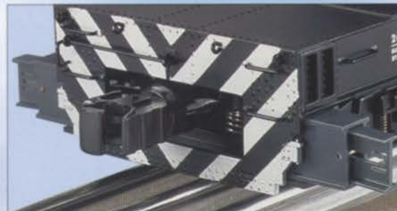
Remotely deployed outriggers and front and rear ElectroCouplers
