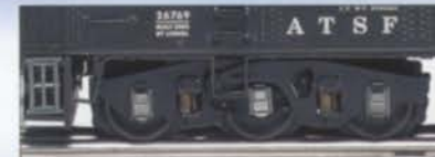
New die-cast metal six-wheel sprung and equalized trucks
