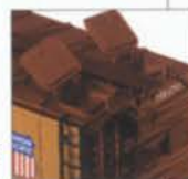
Opening roof hatches
