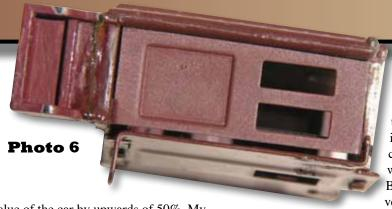
value of the car by upwards of 50%. My opinion is that the flaw has two causes. Clearly, the steps are somewhat exposed. But I feel there must either be some stress in the cast at the point where the top step joins the underside of the vestibule casting
