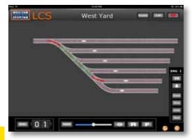
After the track plan was applied to the iPad, they showed how to throw a switch by touching a finger to the screen at the switch icon. The icon changed from a green (straight) to a red (curved) color to indicate the path through the switch. It's reminiscent of the lighted control panels in the command center of the Starship Enterprise. Lt. Commander Data would love this device! Similar actions turn on block sections and action accessories.
