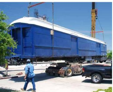
Ironically, the baggage car was moved from Fort Worth to Grapevine – a 20-mile drive – on a flatbed truck, not by rail. A crane lifted the baggage car off its trucks, set it on the flatbed truck, and later reset the car back on its trucks at a section of track prepared in advance in Grapevine. Club members helped lay the rails and spread the ballast for that track section.
