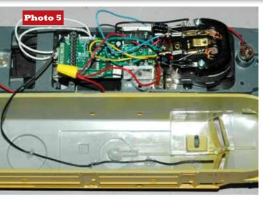
this case it is the perfect solution. I simply applied several dabs to secure the wire as seen in **photo 5**. I made sure to allow enough wire so that I could remove the shell and lay it down next to the loco.
