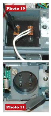
also need to cut a small rectangular hole for the slider of the switch. For the Alco, I decided to the place switch next to the Program/ Run switch. That switch was mounted to a plastic which plate was easily removed. Photo 10 shows the installed switch. As you can see, I needed to
