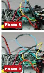
result can be seen in **photo 8**. The blue and yellow wires are the ones from the motor. I was then able to slide the heat shrink tubing over the connection and using a heat gun, shrink it tight, as seen in **photo 9**.
