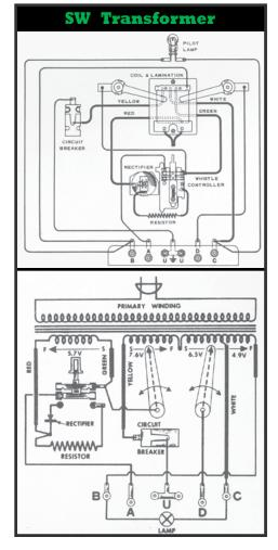
roller is left at a specific setting to supply a "fixed voltage" to a circuit with a current draw more than one amp, over a period of time the carbon roller will harden and deteriorate since the electrical path through it would never change. For transformers with carbon rollers it is a good practice to "zero" all fixed voltages when the layout is not in use and reset them each time one powers-up the layout. I suggest varying the setting by +/-.5 volts.
