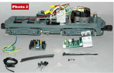
1994 Union Pacific Alco and **photo 2** shows it with its shell removed along with the parts included in the AC Commander kit. The board already on the loco is the electronic E unit that came installed on it. In addition to items supplied in the kit, you'll need some basic tools – a soldering iron, jeweler's screwdriver, wire strippers, etc.
