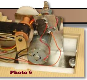
The reason for the larger package was so that the operation of the belt would be automatic. The larger package would activate another micro-switch that would cause the belt to stop automatically. This micro-switch was
