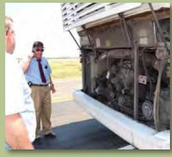
As we left the BEP, a warning beeper sounded on our bus. The driver pulled to the side of the road and discovered that one of the motor belts was shredded. Fortunately, he had a spare belt, and one of our conventioneers, a mechanic, offered to help install it. After a short
