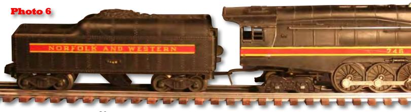
But the wheelbase is different. So is the part number. It's 221-25 for the NYC loco and 2035-14 or 2036-10 for the others. Photo 5 shows the rear truck on a #221 and #2035 for a view of the difference in wheelbase on what initially seemed to me to be a pretty-muchidentical part. The entire motor assembly, drive rod, and front truck also have unique part numbers that don't ever seem to have been used on other locos. Go figure.
