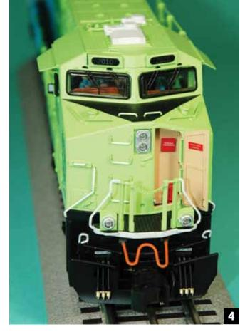
position. **Photo 4** shows the open access door at the front of the loco. The entire body of the loco is diecast, so it is electrically grounded to the frame. For this reason, plastic stanchions were used to support the metal railing that also serves as the antenna to receive Command Control signals.
