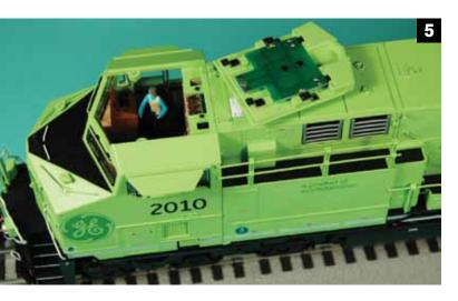
Other details include separately applied builder's plates and radiator vents. The cab openings have windows that can slide open or closed. A section of the cab roof lifts off for a view inside the cab as seen in **photo 5**. The lighting mounted within this roof panel disconnects via sprung metal contacts which restore the circuit when the panel is replaced. The cab interior is lighted and features enhanced panel detail.
