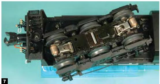
**Photo 7** shows one of the two motored trucks. Notice that the coupler is not attached to the truck. Photo 8 illustrates how the section in front of the truck also pivots, along with the coupler itself.
