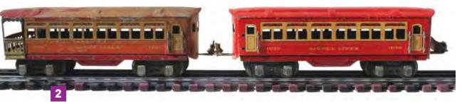
The bodies are one piece: the sides, ends and roof are all one piece bent and tabbed together. Once the car was assembled, it would be
