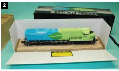
as shown in **photo 2**. Remove the two screws from underneath the board to release the loco.
