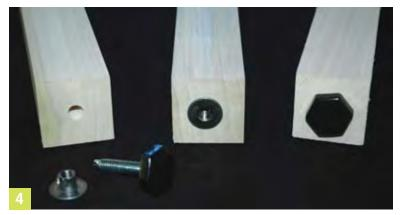
**Photo 4** shows the leg before installation, after the "T" nut is hammered in place, and finally with the leveler installed. The leveler allows an adjustment of up to 1-1/4 inches. The legs in my set were designed to make a table 36 inches high. Legs in several sizes up to 48 inches are available. Additional custom-made sizes are also available.
