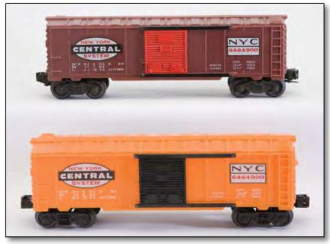
We assume that there are less than a half-dozen examples of these rare boxcars in existence. To avoid the cost of painting, note that these postwar Type IV bodies were unpainted brown and unpainted orange respectively. Furthermore, In lieu of typical heat-stamped decoration and to further reduce production costs, these examples were decorated totally with adhesive emblems for both text and graphics.
