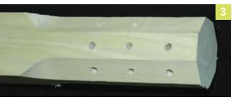
The legs are 1-¾-inch-square poplar wood. The top of each leg has been cut to an octagonal shape as in **photo 3**. The first step is to install "T" nuts into the bottom of each leg.
