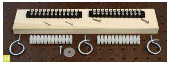
Into the lower edge, Bill secured three metal loops as guides for wires. These loops are open so that wires can easily be added or removed. On the face of the board, Bill added two
