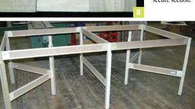
Next, these sub-assemblies are assembled together using more beams to make the outside rails of the top. **Photo 9** shows the construction at this point. Next, more beams are added to the interior parts of the table resulting in a grid of beams to further solidify the benchwork. During this
