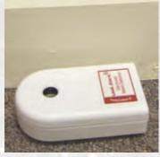
Zircon Leak Alert<sup>TM</sup> Electronic Water Detector leaned against display shelves enclosing the layout tables. Except when being photographed, it lies flat on the floor either on its side or its back so that any moisture would establish a circuit between its two metal strip
