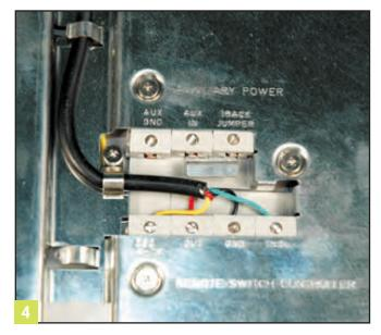
will need to use a small screwdriver to secure the wire into the small terminals. **Photo 4** shows a close-up of the wire terminals. Removing the metal jumper across the two upper terminals converts the switch from track power to auxiliary power. Auxiliary power is connected to the Aux IN and the Aux GND terminals
