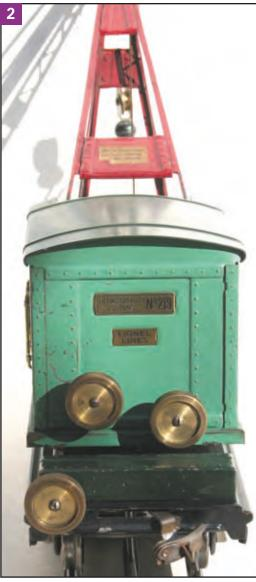
all controlled by the big brass wheels shown in photo 2. The one at the bottom left controls the rig's rotation via a long rod with a worm gear that engages the large spur gear under the car body. See photo 3. The two knobs on the rear of the car body control the hook and the boom through worm and spur gears inside the
