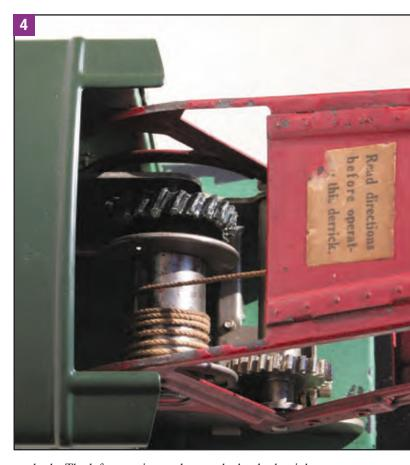
car body. The left one raises or lowers the hook, the right one the boom. See **photo 4** for a look at the gears inside the car body. Notice what big, solid gears they are. They are finetuning knobs; the gear ratios allow slow and precise motion in all three dimensions. No herky-jerky, coarse adjustments. When the big hook is called out to right the loco that spilled off the main, you need fine control. By the way, check out
