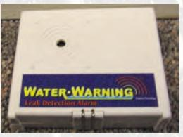
The two parallel metal strips coming out of the case below the label and wrapping around the bottom edge extend across the back of the case (out of sight in this view). Any water saturating the carpet would establish an electrical connection between the metal strips and activate the alarm.
