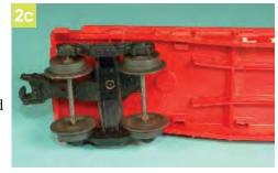
directly riveting the truck to the car, the plate method was abandoned. **Photo 2c** shows the riveted AAR truck.
