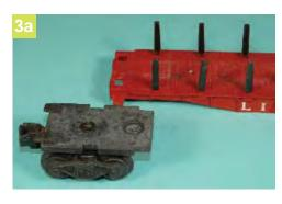
of the car. The opposite end of the plate was secured with a flathead screw through the top of the car. Removing the single screw on the top surface of the flat car allows easy removal of the truck assembly. **Photo 3a** shows the result. The truck was held to the plate through the use of a "C" clip which secured a post riveted to the top of the truck. The undercarriage detail was continued on the die-cast plate. When installed, only the two holding tabs were visible on
