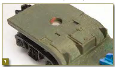
**Photo 7** details the circular area where the plastic AAR truck was riveted directly to the car body. Look closely, and you will notice an area of red that was not completely covered during the painting process.
